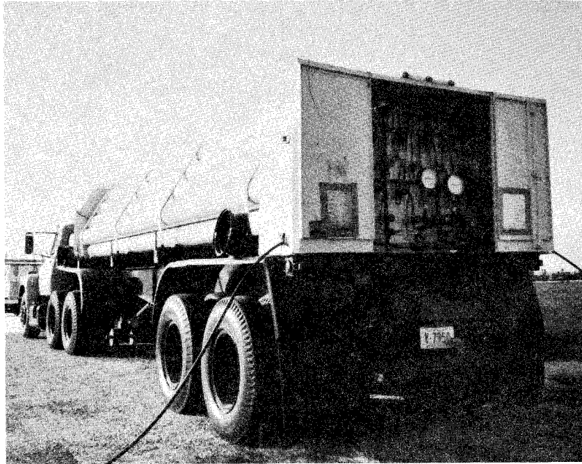
Fig. 1. Lift gases for ballooning are usually transported in cylinders mounted on trailers as shown here. The cylinders are connected at the rear by a manifold in such a way that gas may be taken from any one or any combination of them simultaneously. Each tube normally has its water volume stamped on it.
